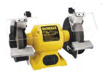
workpiece from being jammed between the wheel and the rest. OSHA also states that the distance between the grinding wheel and the adjustable tongue must never exceed 1/4 -inch. Another useful tool to buy is a Bench Grinder Safety Gauge. Available online for \$19 at www.RockfordSystems.com.
