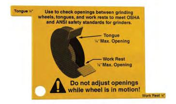
Keep the tools such as an Allen wrench or hex key and a wrench to make the adjustment before EVERY use of the equipment.
